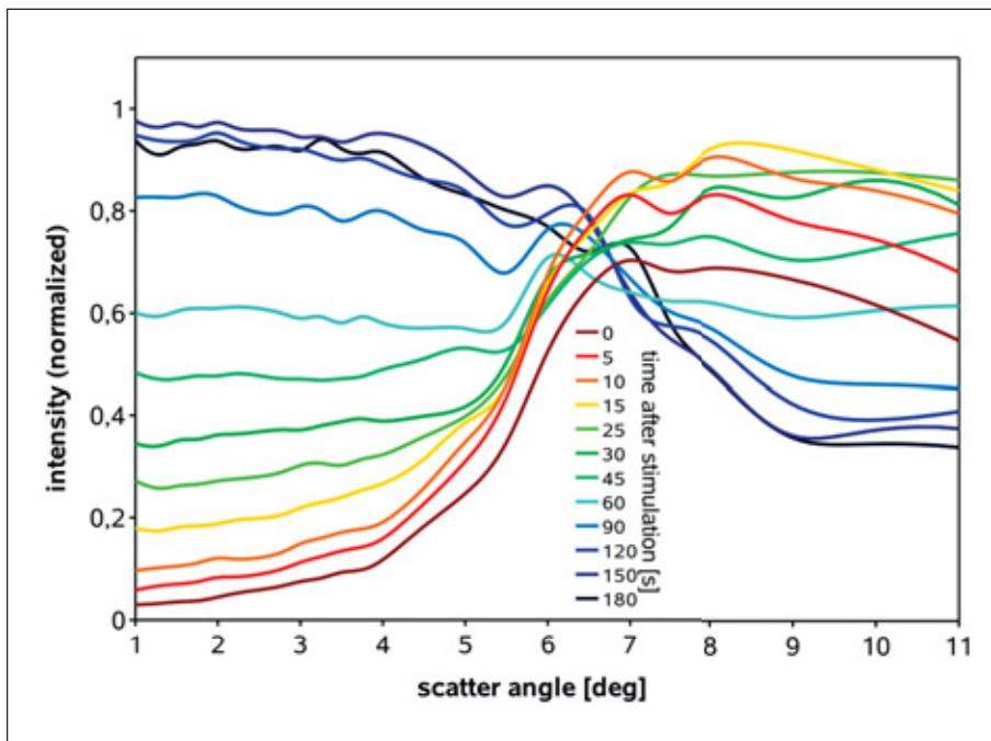
Fig. 2: Changes in the angle-dependent scatter profile of a platelet suspension during the activation process as observed with the LASCA (low angle light scatter analysis) setup.
