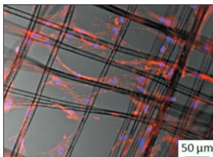
Fig. 3: Cell growth on melt electrospun fibers.
