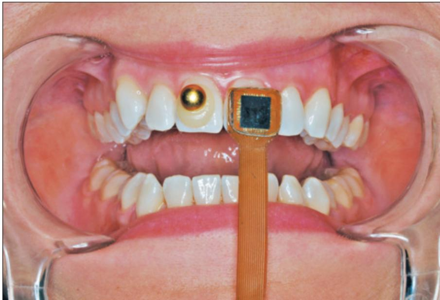
Fig. 2: Novel tooth mobility setup. A spherical magnet is affixed to the left tooth, on the right a hall sender is glued to the incisor thus making measurement of relative motion possible.
